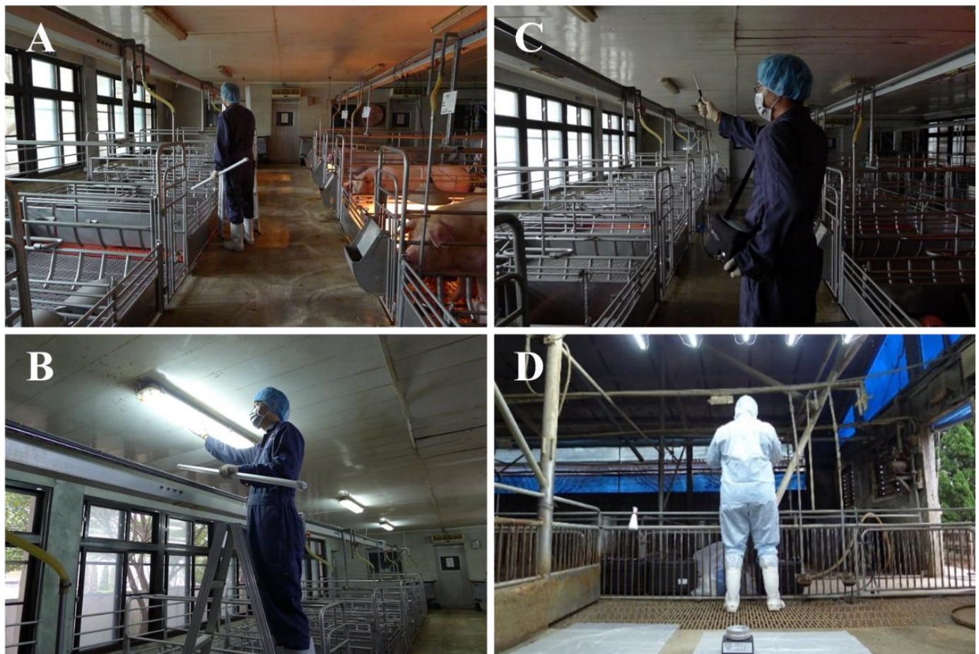
Figure 1: Test of LED device in the SPF pig farm and the traditional pig farm. (A) SPF pig farm. (B) Replace the LED lamp in SPF farm. (C) Erection of LED lamps in the traditional pig farm. White visible LED light was at 450 nm wavelength.
