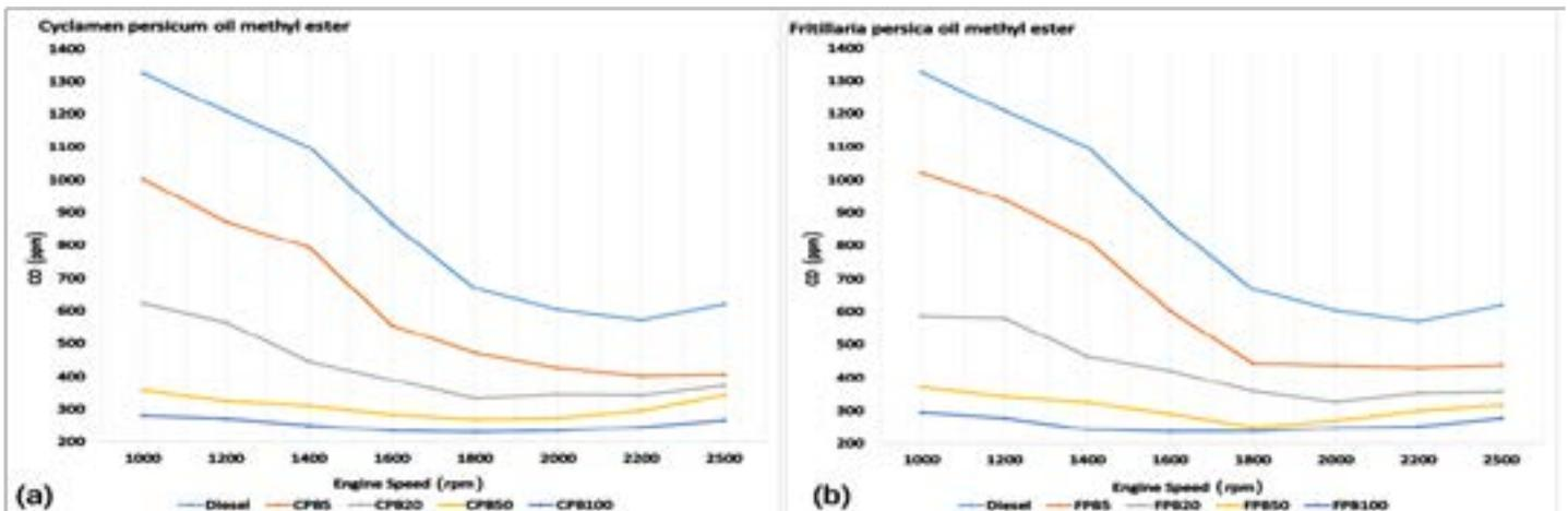
Figure 6: The variation of CO emission at the full loaded engine for the cyclamen persicum oil methyl ester and fritillariapersica oil methyl ester blends and diesel.
