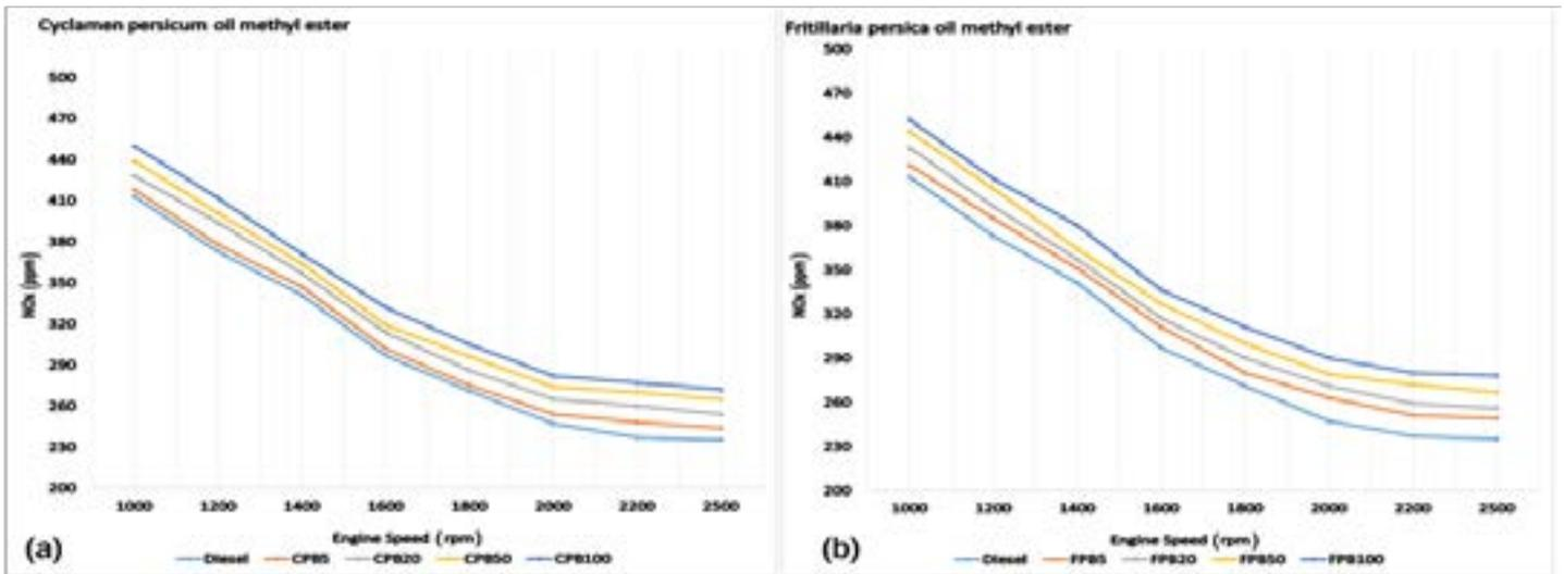
Figure 5: The variation of NOx emission at the full loaded engine for the cyclamen persicum oil methyl ester and fritillariapersica oil methyl ester blends and diesel.
