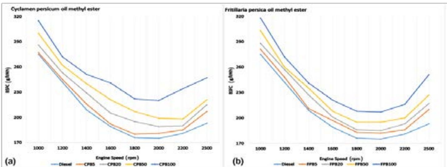
Figure 3: The variation of BSFC at the full loaded engine for the cyclamen persicum oil methyl ester and fritillariapersica oil methyl ester blends and diesel.
