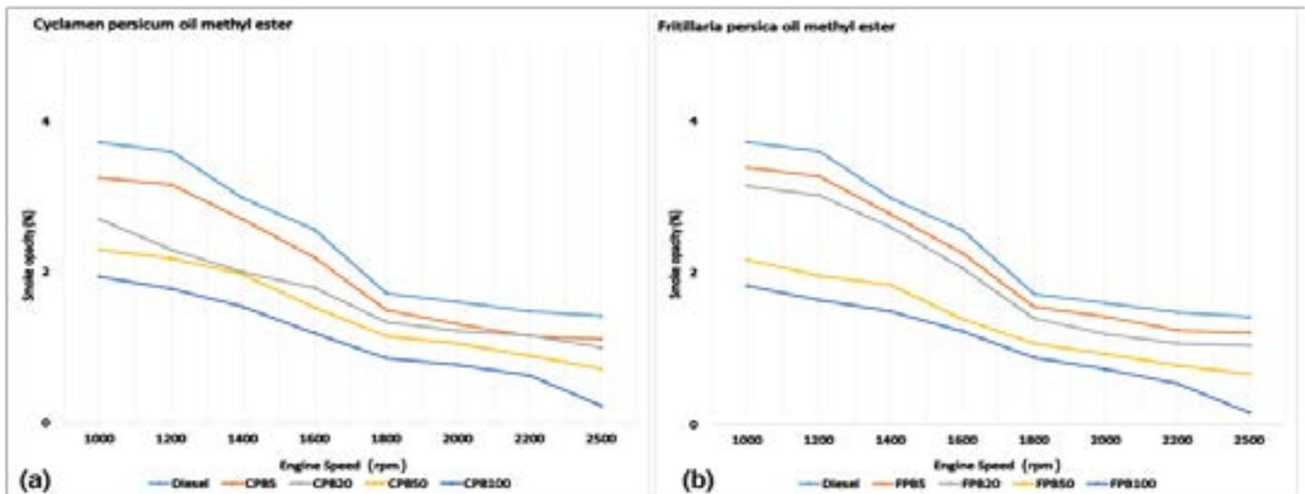
**Figure 8:** The variation of smoke opacity at the full loaded engine for the cyclamen persicum oil methyl ester and fritillariapersica oil methyl ester blends and diesel.
