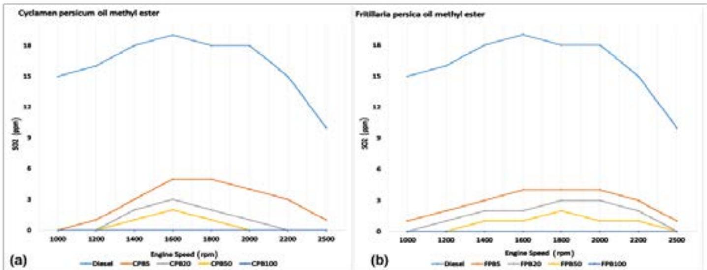
**Figure 7:** The variation of SO<sub>2</sub> emissions at the full loaded engine for the cyclamen persicum oil methyl ester and fritillariapersica oil methyl ester blends and diesel.
