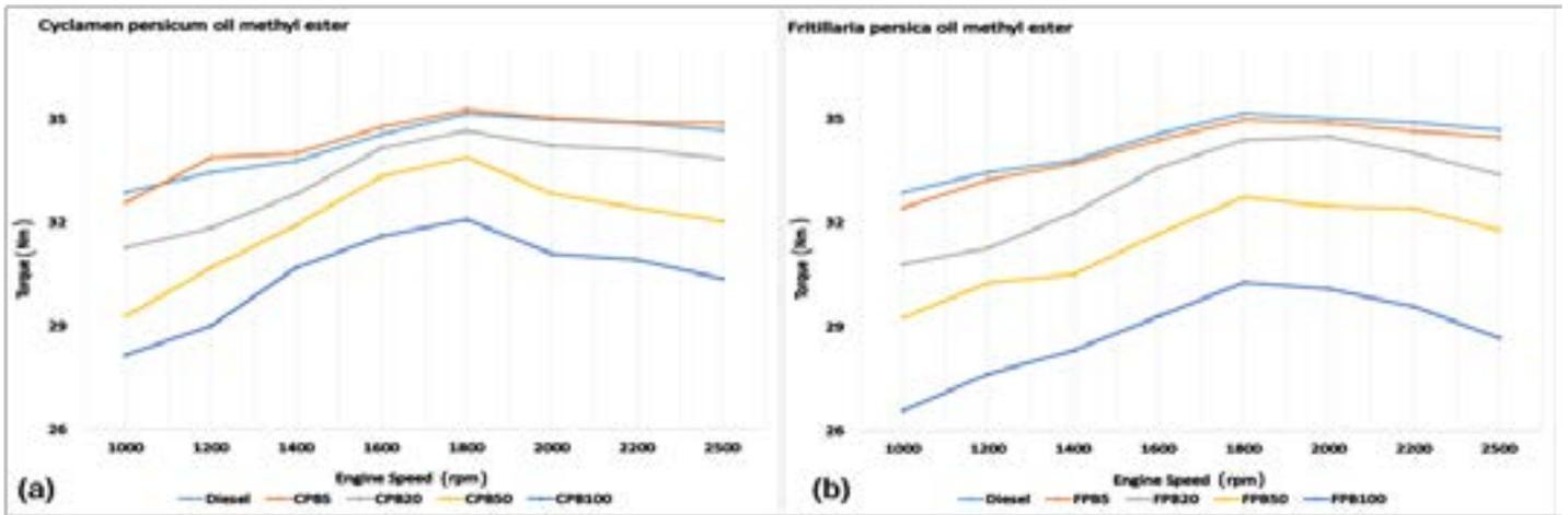
Figure 1: The variation of torque at the full loaded engine for the cyclamen persicum oil methyl ester and fritillariapersica oil methyl ester blends and diesel.
