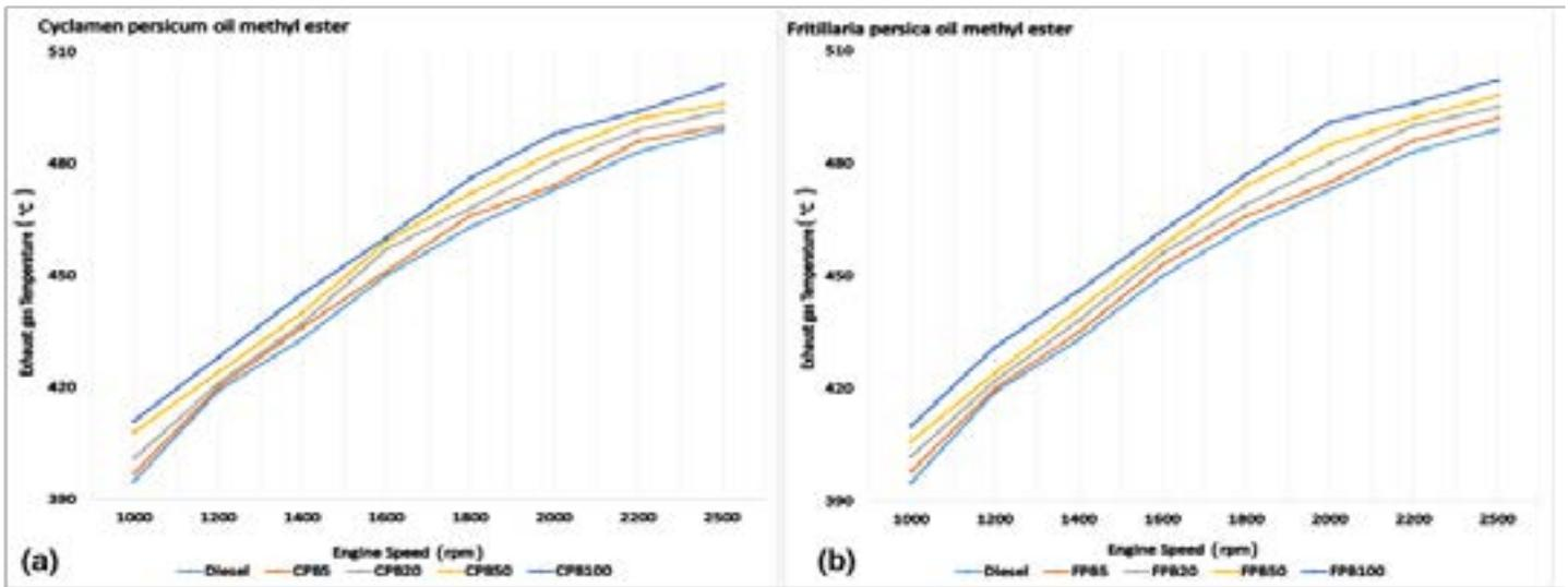
Figure 4: The variation of EGT at the full loaded engine for the cyclamen persicum oil methyl ester and fritillariapersica oil methyl ester blends and diesel.
